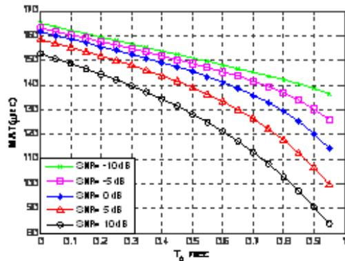
**Fig. 8:** MAT versus pulse waveform width, with different SNR and  $N = 265$ .
