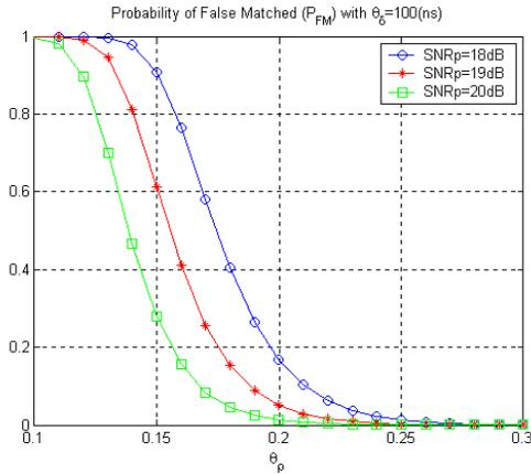
**Fig.3:** Probability of false matched (PFM) with delay threshold ( $\theta_\delta$ ) 100 nsec.
