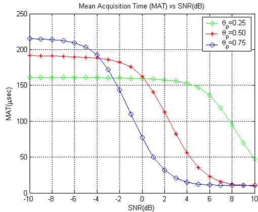
**Fig. 7:** Mean acquisition time for different normalized signal strength threshold values.
