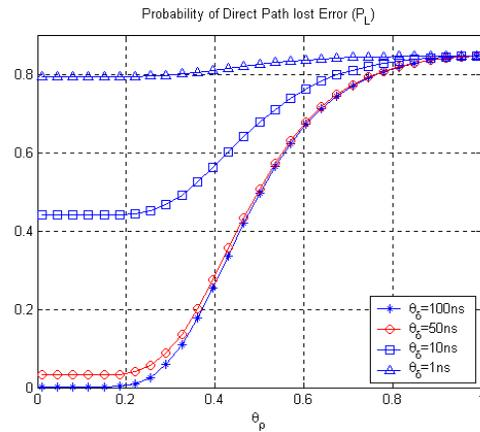
**Fig.2:** Probability of a direct path lost error (PL) with a peak SNR of 18 dB.
