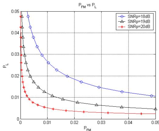
**Fig.5:** False matched probability versus probability of direct path lost for different peak SNRs.
