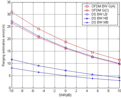
**Fig.1:** Ranging error based on the CRLB for various types of UWB IEEE802.15 standards.
