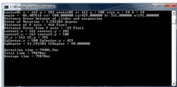
Fig. 7: The report shows misalignment in x - y plane and the rotation above z axis.
