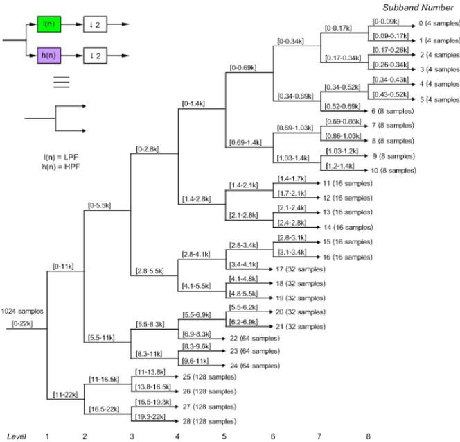
Figure 3 Decomposition Tree for 44.1kpbs Audio Frame
