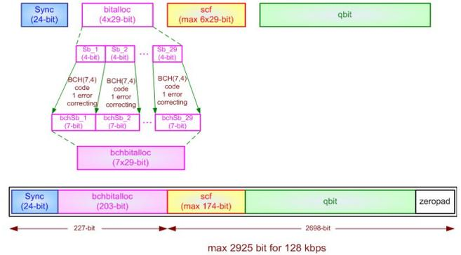
Figure 4 Frame Structure of Wavelet-Packet Audio Coder
