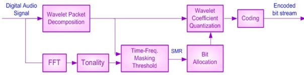
Figure 2 Structure of Wavelet-packet Audio CODEC
